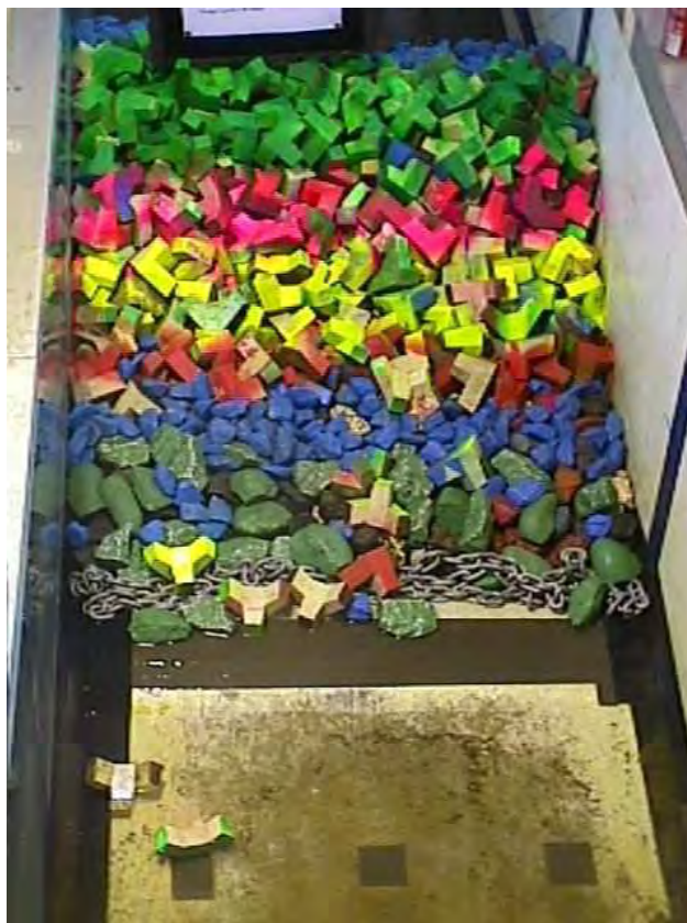
(b) Damage to two-layer Hanbar primary armour after 2000 waves
