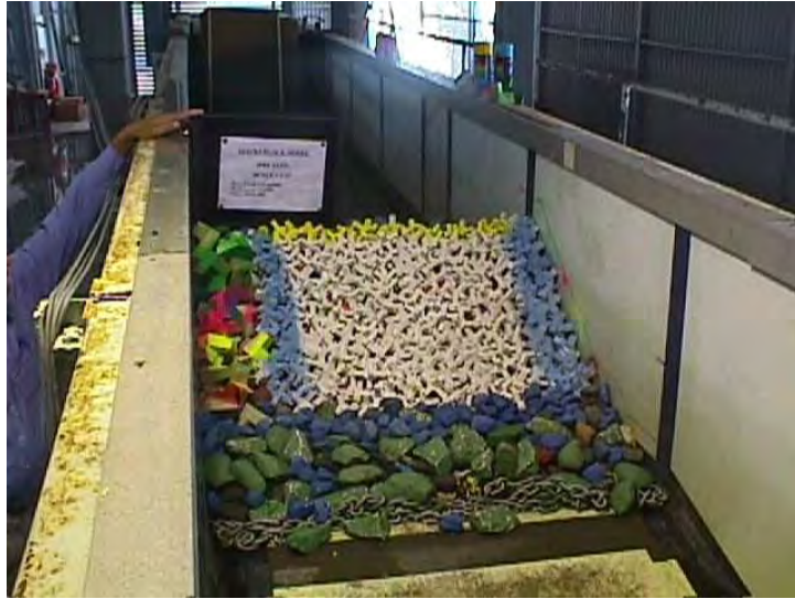
(a) Ajacks with Hanbar and Stubby interface - before testing
