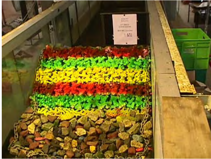
(a) Stubby armour units before testing
