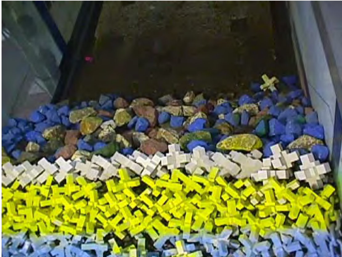
(a) Minor damage to crest when using the Stubby unit for crest protection H_s = 4.5 m, T_p = 8.05
