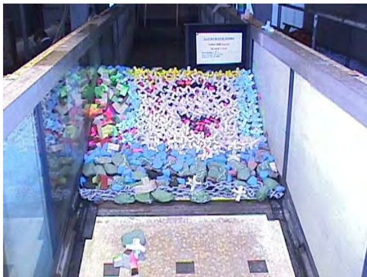
(c) Damage to cross-section after 2000 waves H_s = 4.5 m, T_p = 8.0 s
