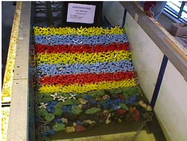
(b) Ajacks cross-section with bundled toe units after 2000 waves H_s = 4.5 \text{ m} , T_p = 8.05
