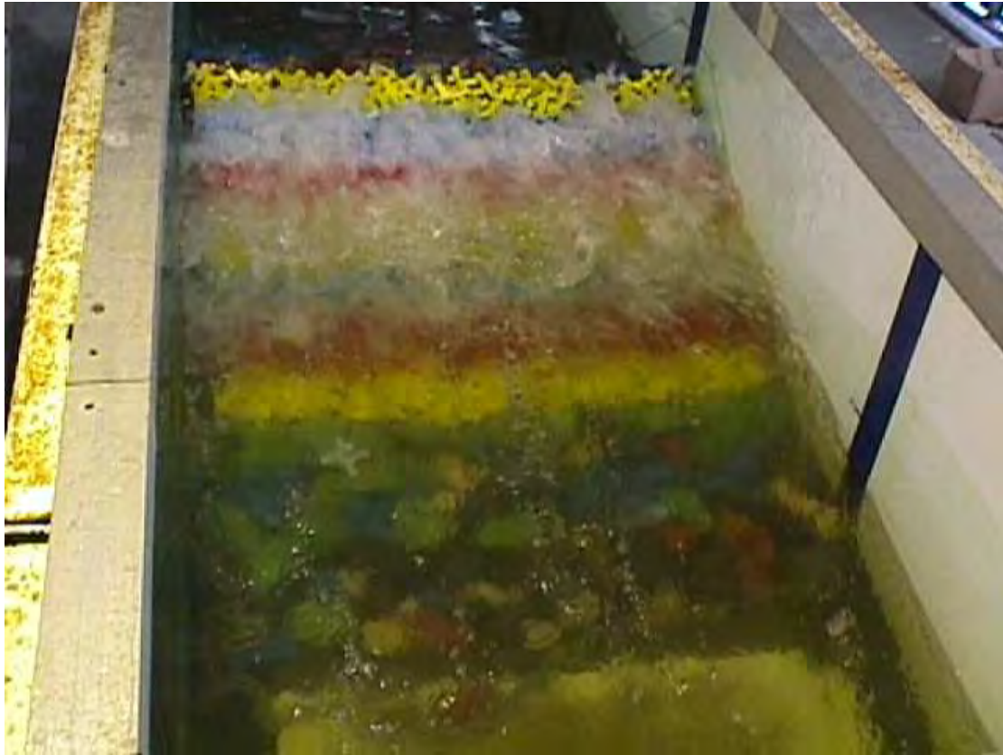
(a) Wave about to overtop crest H_s = 4.5 \text{ m} , T_p = 8.0 \text{ s}
