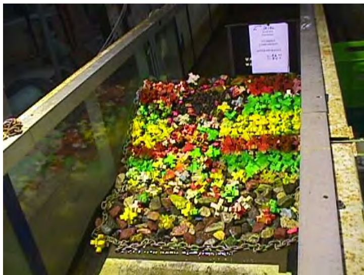
(c) Ajacks armour - damage after 500 waves H_s = 5.6 \text{ m} , T_p = 8.0 \text{ s}
