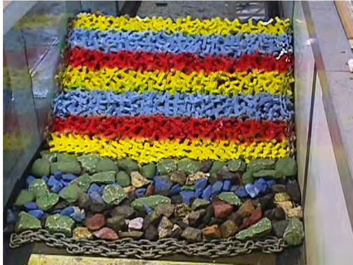
(a) Ajacks cross-section with bundled toe units prior to testing
