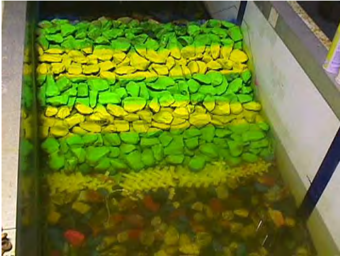
(a) Two-layer stone armour with Ajacks toe before testing
