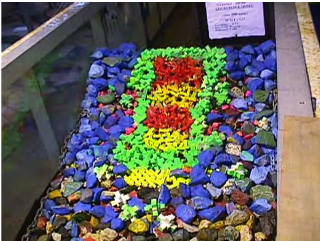
(b) Damage to stone interface after 2000 waves. The Ajacks armour was undamaged H_s = 4.5 m, T_p = 8.0 s
