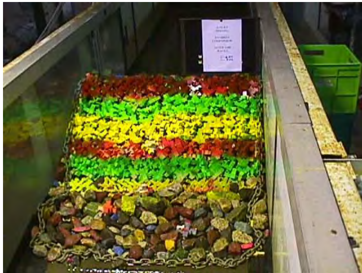
(b) Stubby armour - after 2000 waves four units displaced H_s = 4.5 \text{ m} , T_p = 8.0 \text{ s}
