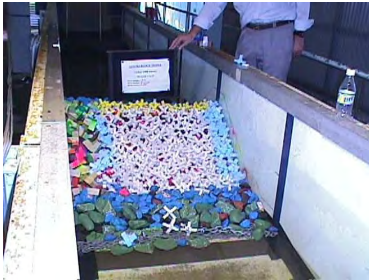
(b) Damage to cross-section after 1500 waves H_s = 4.5 m, T_p = 8.0 s
