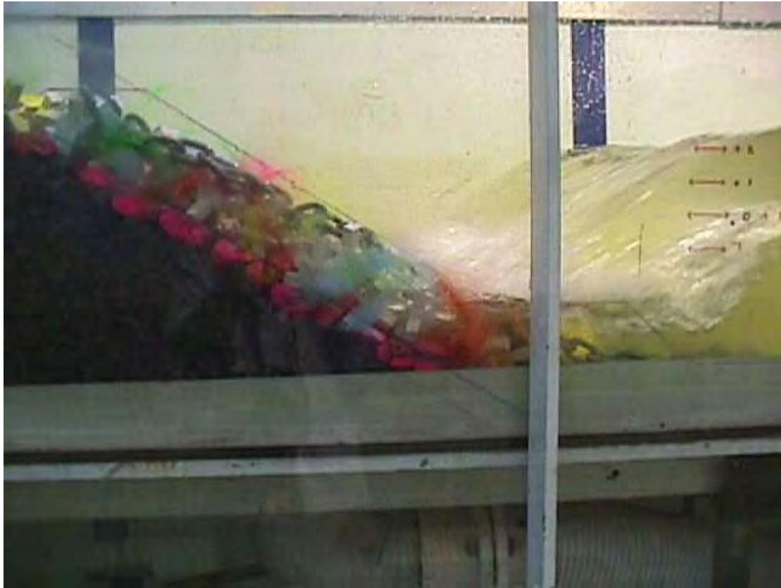
(a) Wave plunging on toe of cross-section H_s = 4.5 m, T_p = 8.0 s
