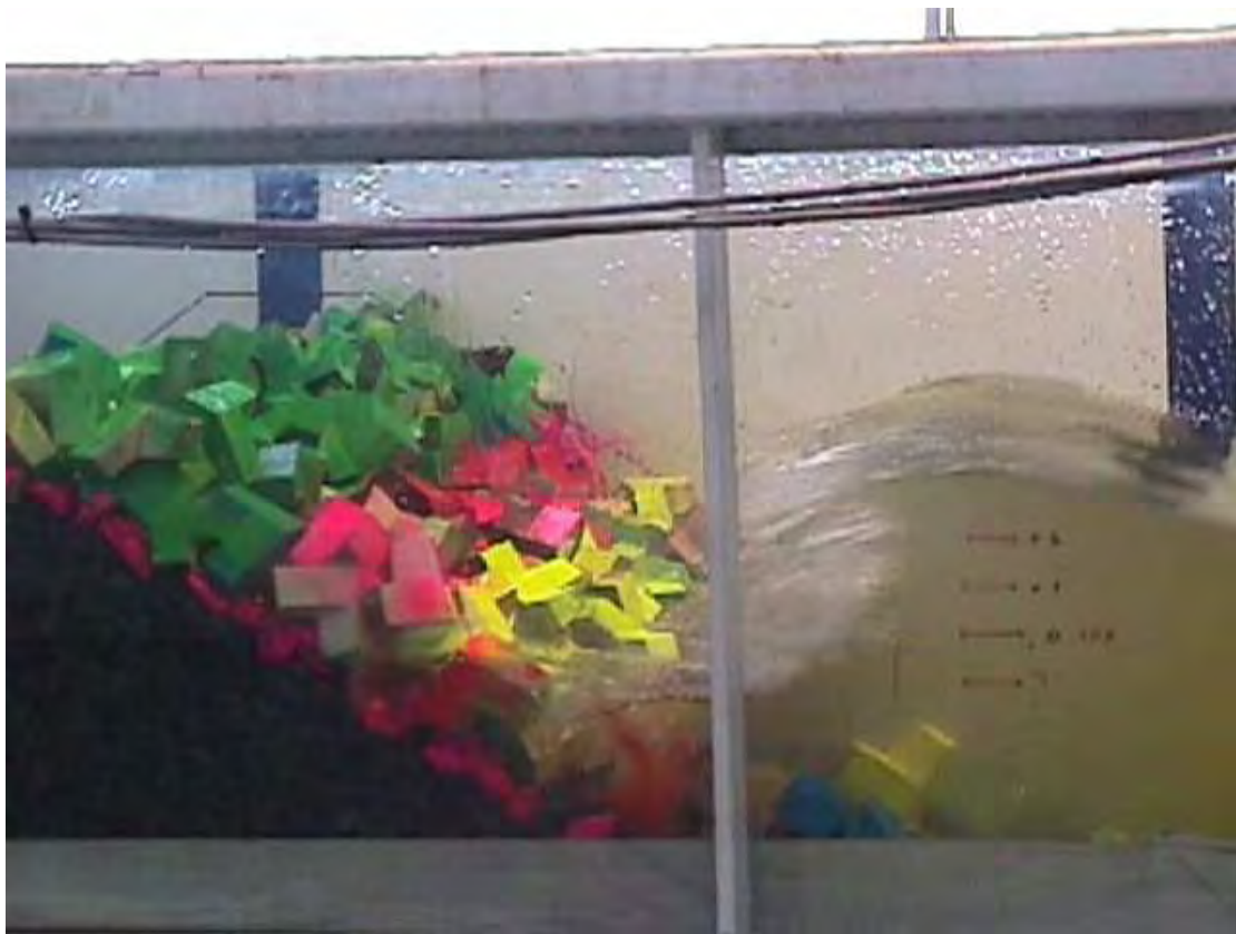
(a) Wave plunging on two-layer Hanbar primary armour H_s = 4.5 m, T_p = 8.0 s
