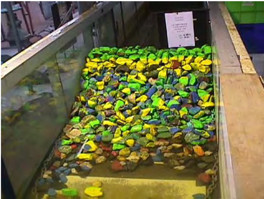
(b) Damage to stone armour after 2000 waves H_s = 4.5 m, T_p = 8.0 s
