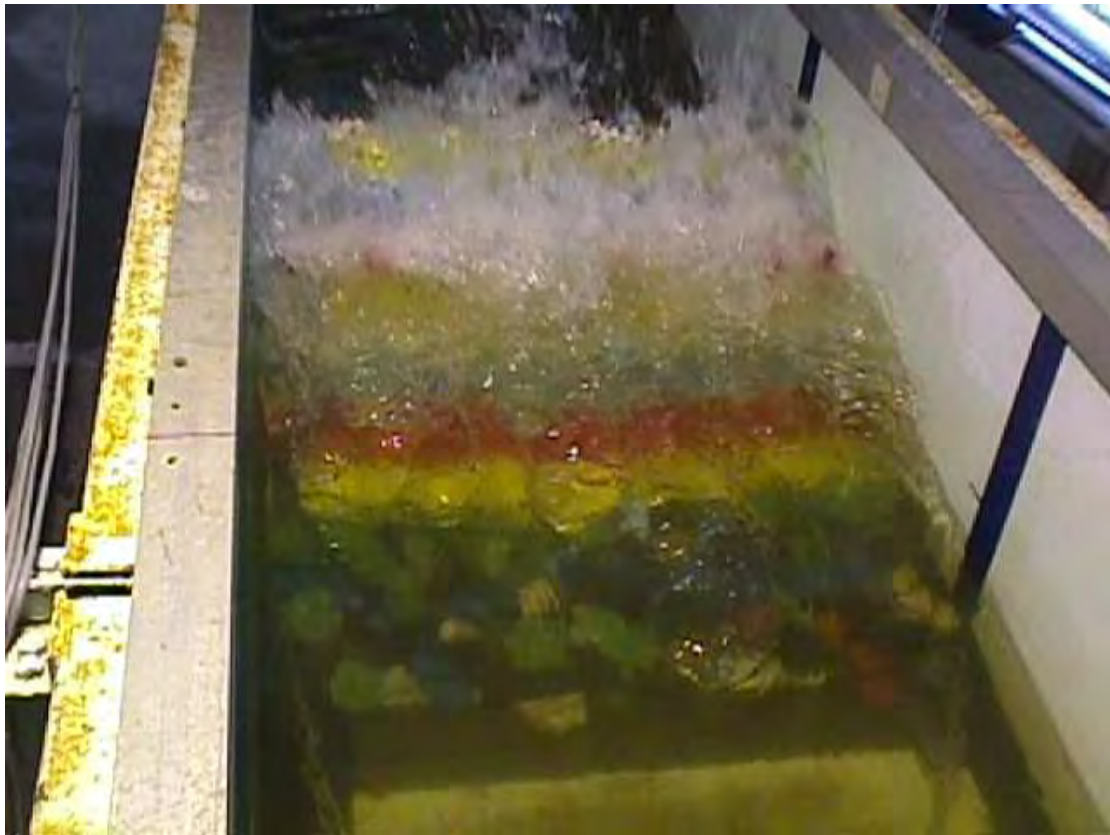
(b) Extensive wave overtopping of cross-section
