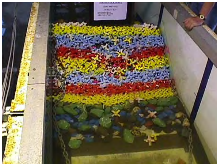
(c) Damage to cross-section after 500 waves H_s = 5.6 \text{ m} , T_p = 8.05
