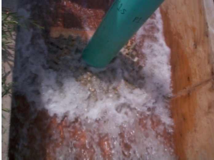
Figure 3.5a. Stability test of 5x4x5 A-JACKS modules, unsubmerged conditions. Note flow shedding around protected pier.
