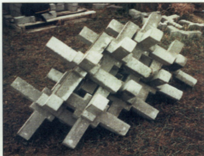
Left: This FiberDam product, which is black geotextile fibers, was placed behind the A-Jacks in order to prevent losing any backfill material back into the channel. Right: The A-Jacks product was utilized instead of rip rap to control the erosion in the Beals Slough project. Andy Bailey, with the Lower Platte River South district, said this was the first application of this product in the area.
